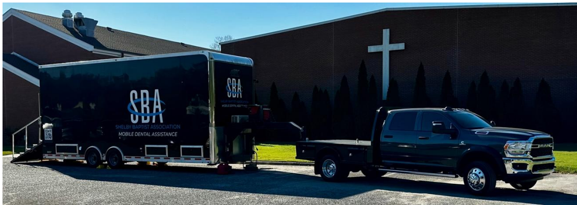
Unit Dimensions: Box=28 ft. (37 ft with gooseneck); Truck = 19.2 ft; Total length=52 ft
